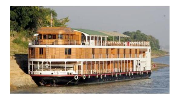
The RV Paukan is modeled after the steamers designed by the Scots engineers and built in the shipyards of Glasgow. The trick is to produce as big a boat as possible with as shallow a draft as possible. The Paukan draws 1.5 meters, or a tad under five feet of water. There are boats as big on the Irrawaddy now with even shallower drafts.
